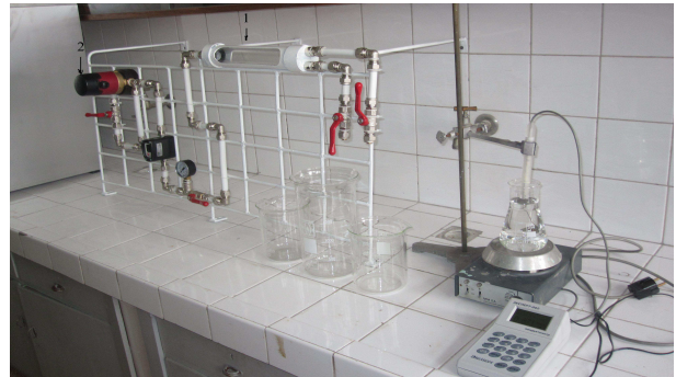
Fig. 4 Laboratory installation for the separation of emulsions using fractal systems
