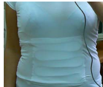
Fig. 4 Knitted shirt with optical fiber sensor
