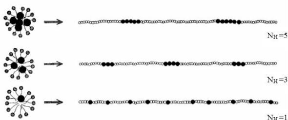
Fig. 2 Different N_H values reflect different arrangement of hydrophobic monomers on the polymer chain (Excerpt from [14])
