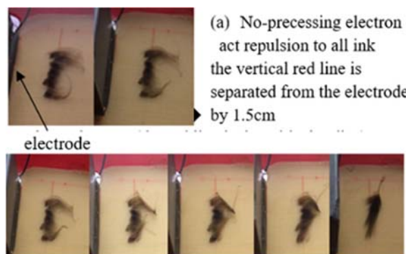
Fig. 3 The screenshots of the experimental video as B is 0.12 T and r_c is 1.5 cm
