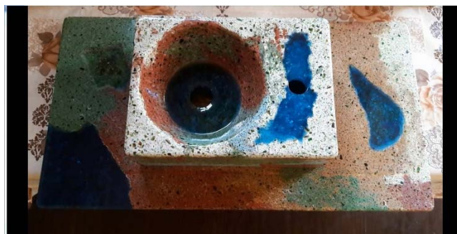
Fig. 9 Prototype Bathroom Sink and Counter Top
