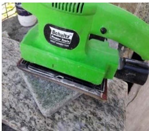
Fig. 8 Polishing with Sander Machine
