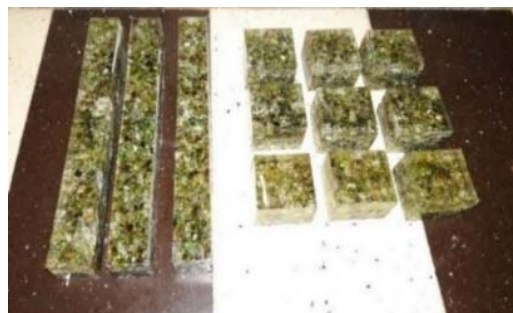
Fig. 3 R2: 50% Glass, 100 g Polyester Resin, 2 g Catalyst
