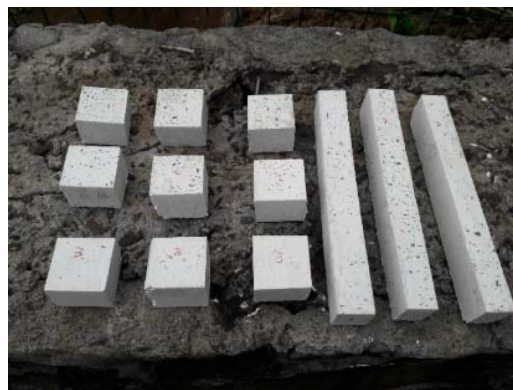
Fig 2 C2- 50% Glass, 100g Cement, 100 ml Water
