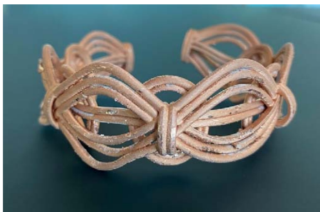
Fig. 6 3D printing in copper of the S/S 2003 bracelet - Galvanised Bronze Brass - File ID 50720 with the FDM and BMD Desktop Metal 3D technology
