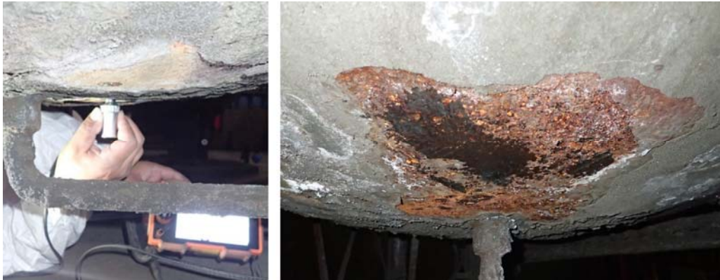
Fig. 3 Measurements with the DMS Go instrument used in non-destructive testing
