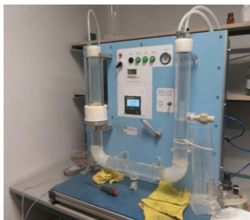
Fig. 4 Experimental device for permeability normal to the plane test according to [22]
