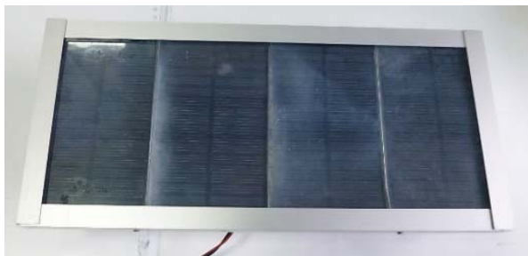
Fig. 4 Photovoltaic conversion system
