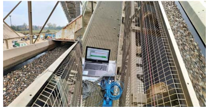
Fig. 6 Sound and vibrations recorded on conveyor belts using microphones and accelerometers
