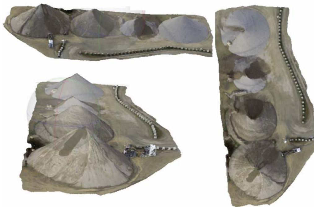
Fig. 3 Reconstruction of the volume of the stockpiles using images taken by drones
