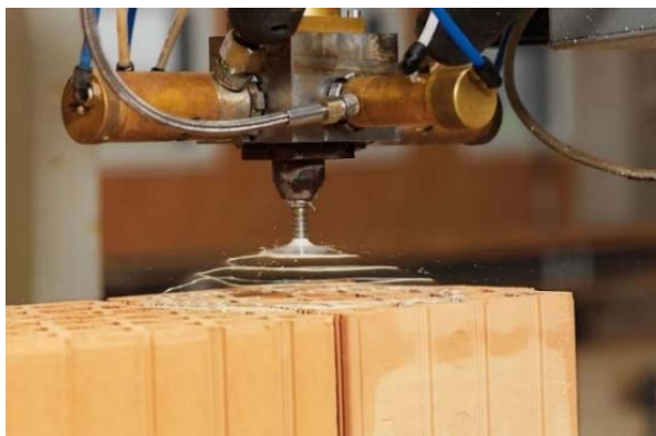
Fig. 2 Application of the two-component adhesive in the precast plant [4]
