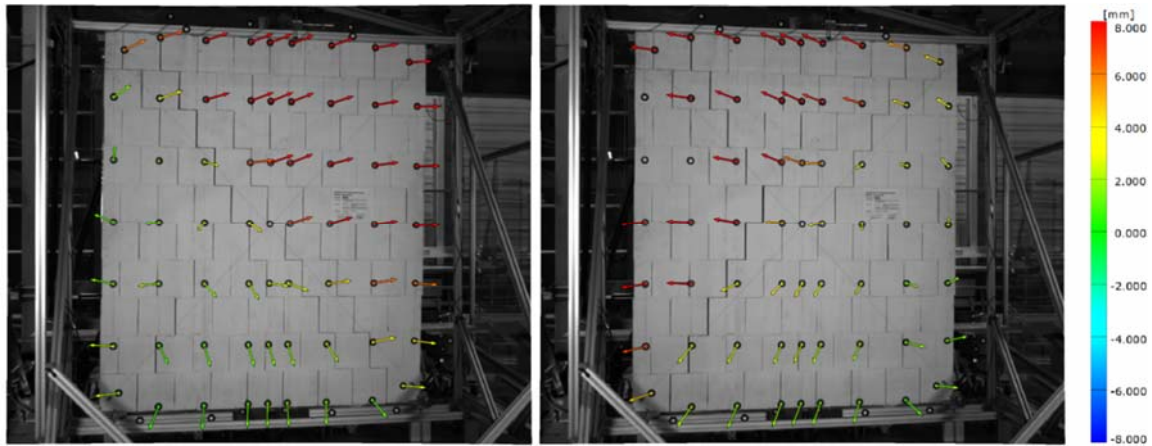
(a) W3: Displacements of wall surface at minimum negative horizontal force and Displacements of wall surface at maximum positive horizontal force
