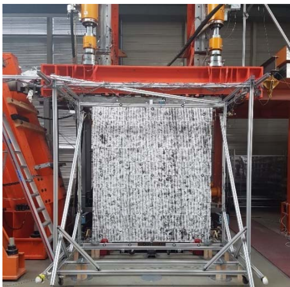
Fig. 3 Test setup: test wall
