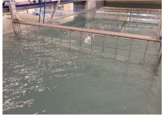
Fig. 8 Photo of the welded mesh panel affixed to the downstream face of the aluminium frame; the shallowest submerged horizontal bars can be seen just beneath the free surface
