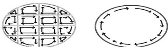
Fig. 12 Internal structure of a magnet
