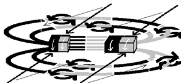
Fig. 28 Magnetic lines approaching by opposite poles
