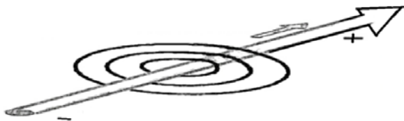
Fig. 6 Side perspective of magnetic waves formed by current electric cable
