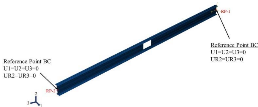
Fig. 4 Definition of boundary conditions for the stress analysis model
