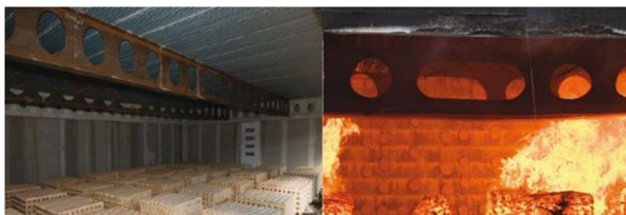
Fig. 1 Fire tests on long cellular beam as isolated and integrated beam in frame structure [16]
