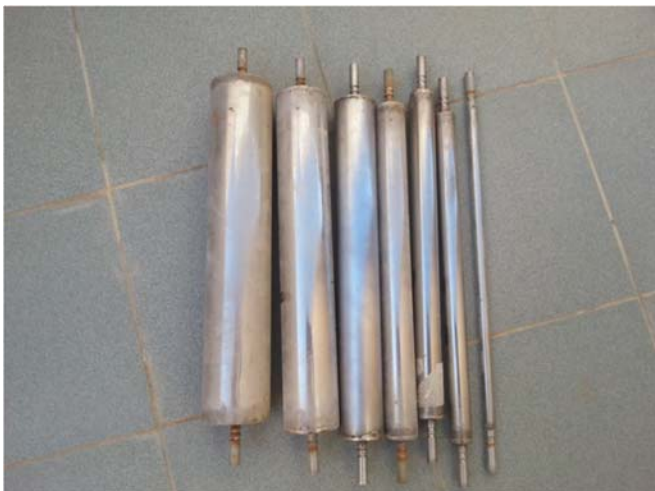
Fig. 5 Cylinder with Different Outer Diameters (from Right to Left 13 mm, 25 mm, 38 mm, 51 mm, 64 mm, and 76 mm with a length of 400 mm)
