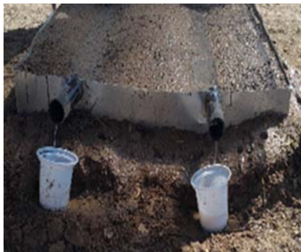
Fig. 2 Runoff and sediment collecting equipment at the out let of the plot
