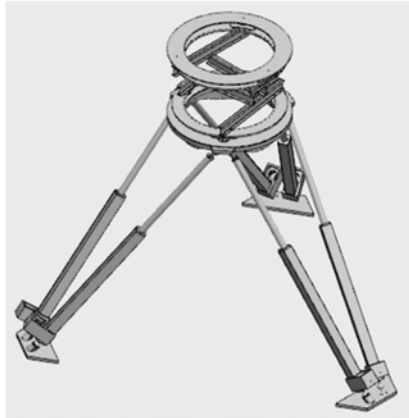
Fig. 2 Simplified Stewart Platform Mechanical Drawing
