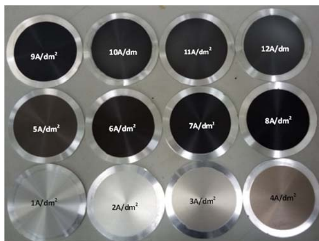
Fig. 2 The images of 6061 aluminum alloy after anodization under the conditions of 1~12 A/dm 2 , 50 cm 2 , 22 °C, 2 0 min
