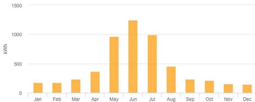
Fig. 7 The average solar system monthly production at the selected location in Tucson
