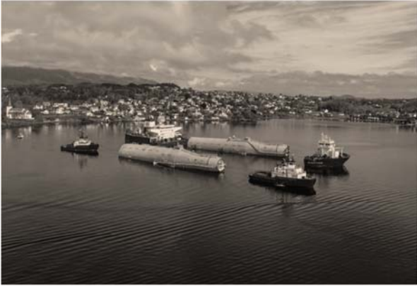
Fig. 9 Heavy transport vessel float off [16]
