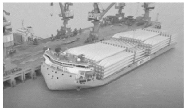
Fig. 29 Heavy transport vessels with blades [41]
