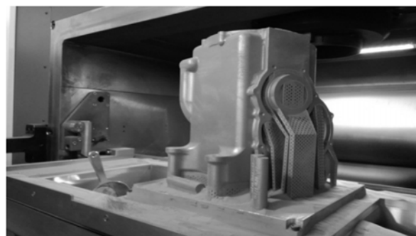
Fig. 9 Prototype of a GTE gearbox housing, made from AlSi10Mg alloy powder
