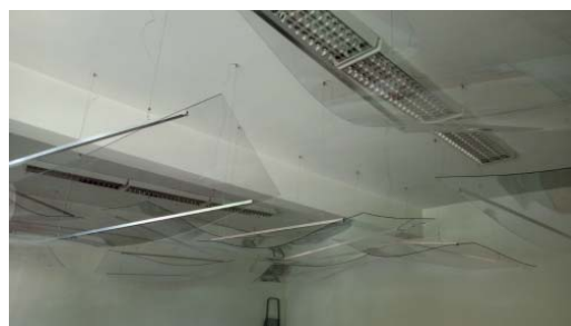
Fig. 2 Reverberation room in UACG according EN ISO 354
