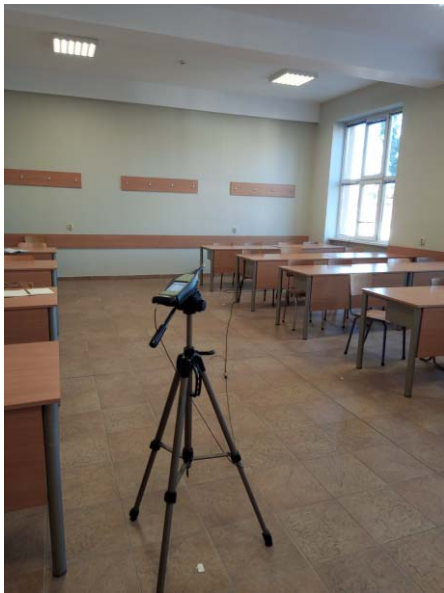
Fig. 3 Photograph of the classroom during measurement of the reverberation time
