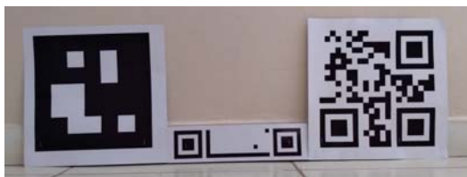
Fig. 11 Markers with sizes to be detected at 10 m distance
