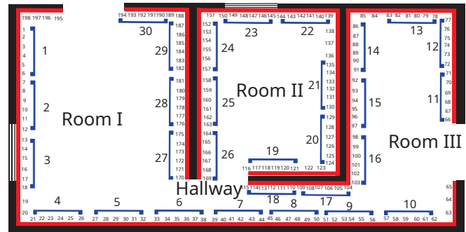
Fig. 4 Example of a floor plan containing the tape (in red) for each room with their respective CM codes. The blue square brackets show the TMs formed by a set of 6 CMs
