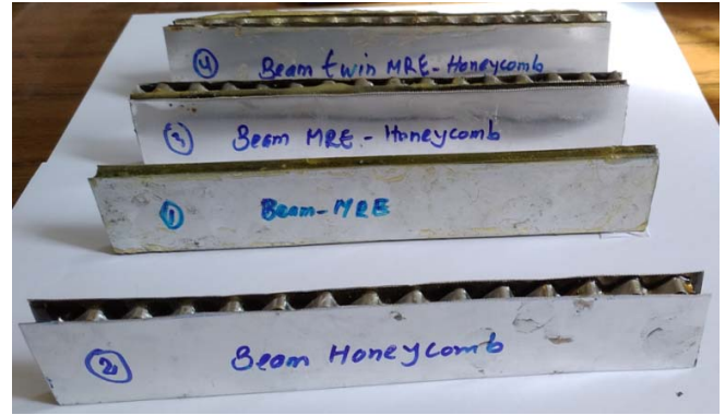
Fig. 2 Different elaborated specimens, (1) MRE beam, (2) Honeycomb beam, (3) MRE Honeycomb beam, (4) twin MRE-Honeycomb beam
