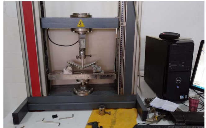
Fig. 3 Three-point bending test, Instron 8561 universal testing machine
