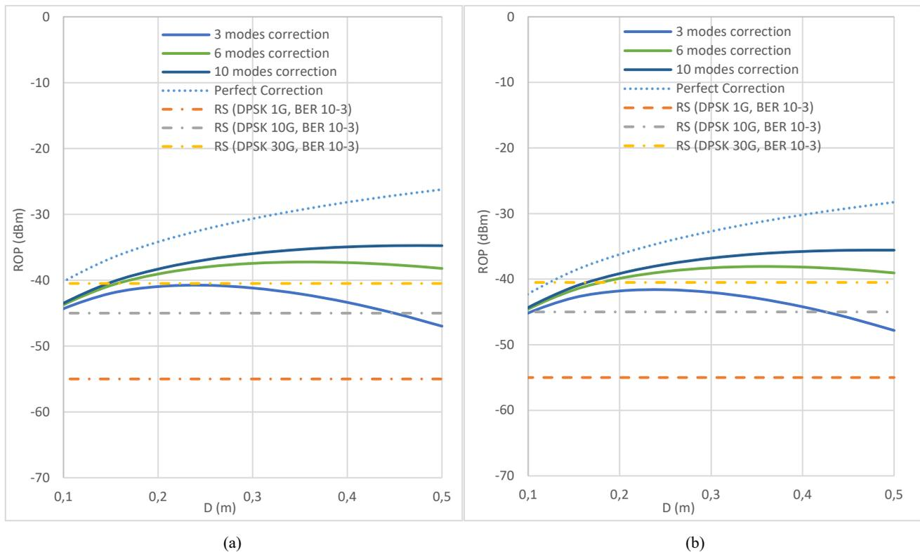
Fig. 4 Received Optical Power ROP (dBm) as function of the receiver telescope diameter  $D$  (m): (a) LEO to ground link case; (b) MEO to ground link case
