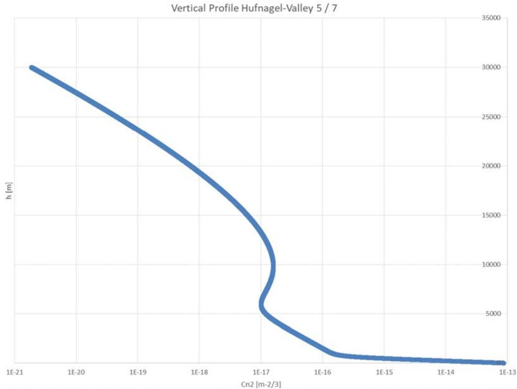
Fig. 1 Worst Vertical turbulence profile according to Hufnagel-Valley model; Averaged wind velocity: 15 m/s; Turbulence Structure function at the ground reference  $C_n^2(0) = 8.7E - 14 m^{-2/3}$
