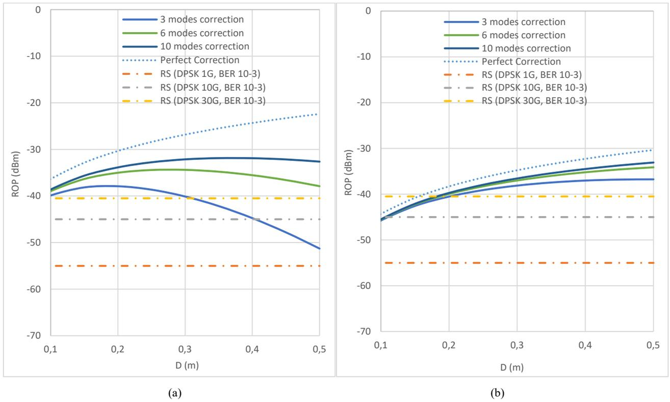
Fig. 2 Received Optical Power ROP (dBm) as function of the receiver telescope diameter D (m): (a) Horizontal link at 500 m, (b) Horizontal link at 150 m
