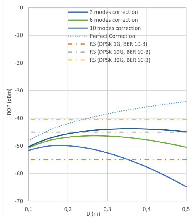
Fig. 5 GEO to ground link case: Received Optical Power ROP (dBm) as function of the receiver telescope diameter D (m).
