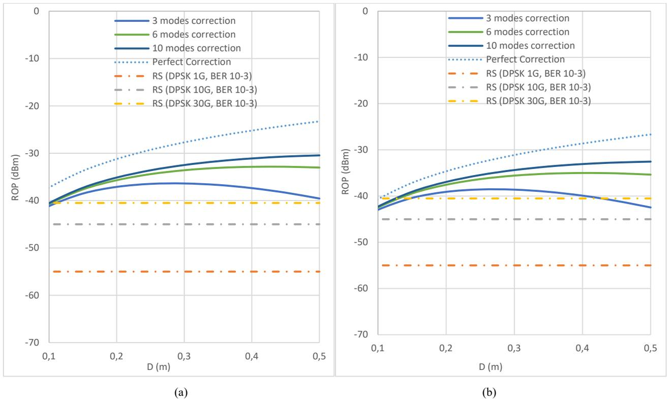
Fig. 3 Received Optical Power ROP (dBm) as function of the receiver telescope diameter D (m): (a) Aircraft to ground link case; (b) HAPS to ground link case
