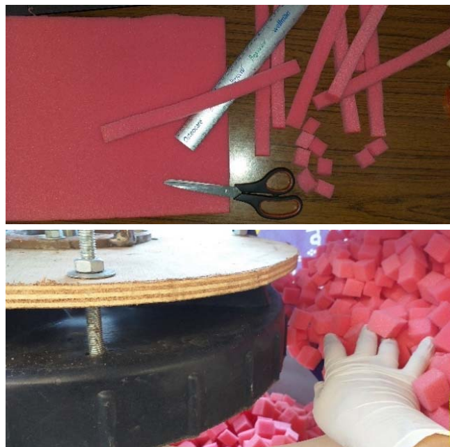
Fig. 6 Preparation of the bio-media and filling of the reactor
