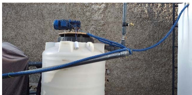
Fig. 5 Manufacture and assembly of mechanical agitators
