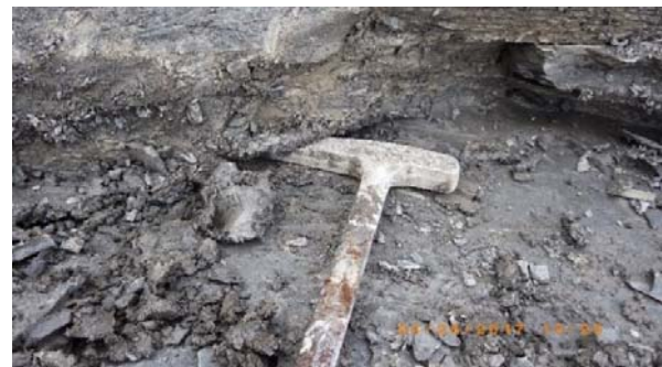
Fig. 3 BP25 with approximately 20 mm of clay gouge infilling
