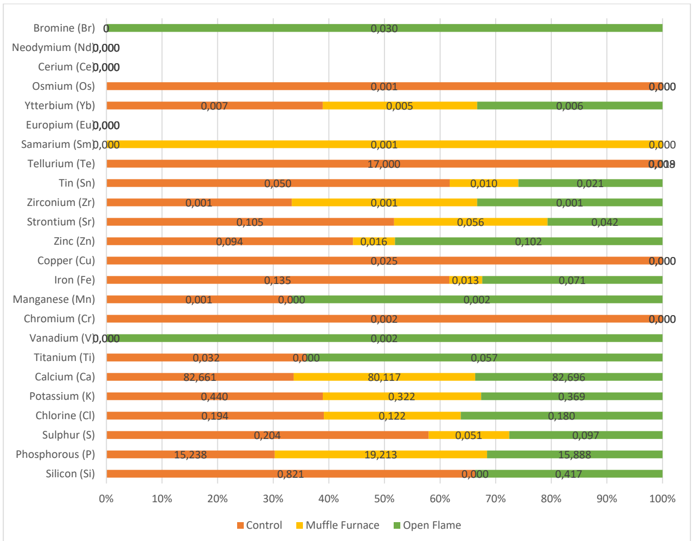
Fig. 8 XRF results showing the concentrations of minerals in each sample
