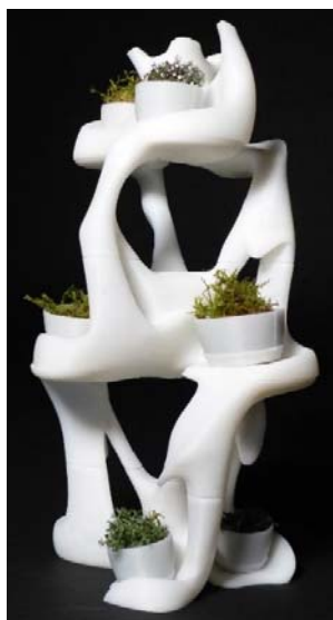
Fig. 8 3D printed prototype of column structure
