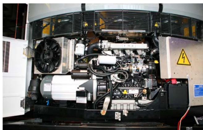
Fig. 1 Transport refrigeration power pack unit for thermal analysis
