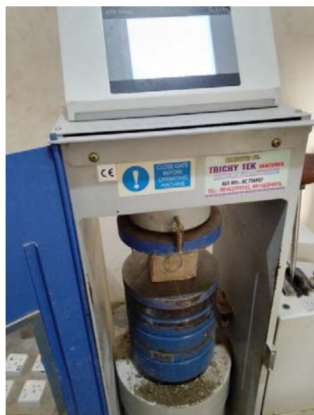
Fig. 6 Compressive strength testing of samples
