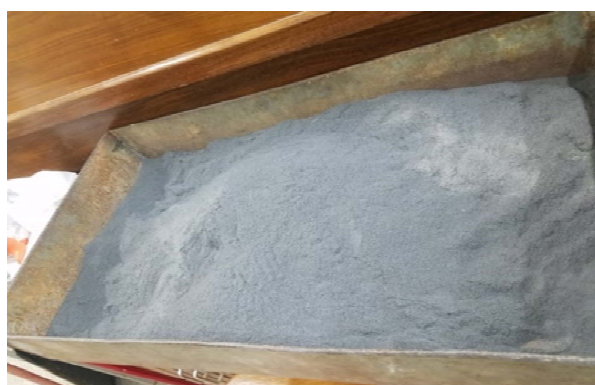
Fig. 2 Calcinated and milled RHA
