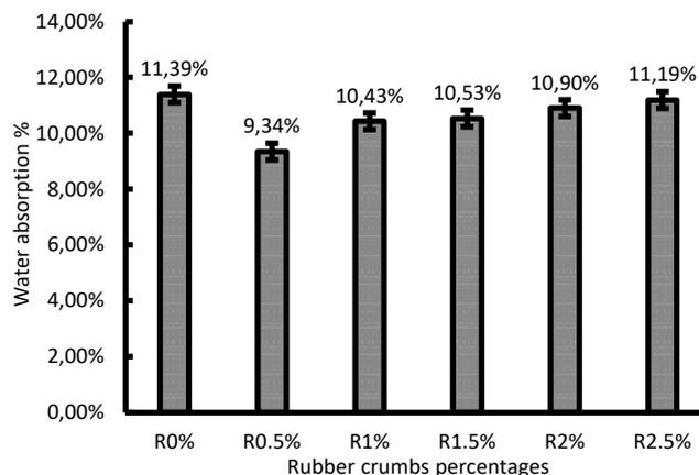
Fig. 4 Water absorption results
