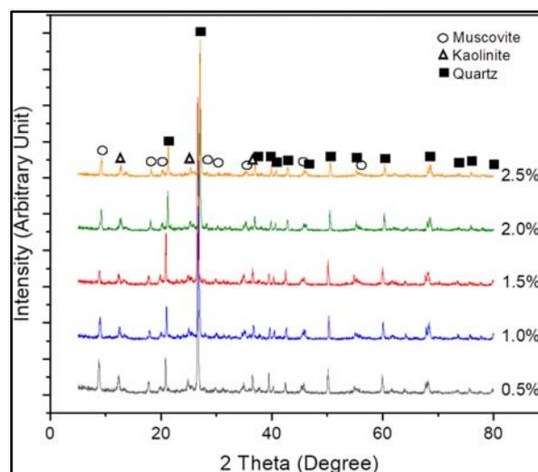
Fig. 2 The XRD pattern of samples with various crumb rubber percentages ranging from 0.5 wt.% to 2.5 wt.%
