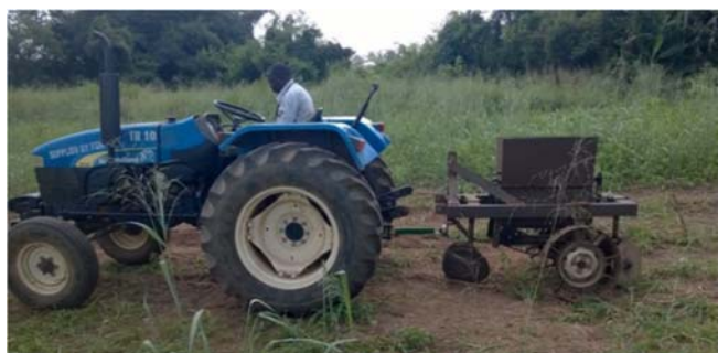
Fig. 1 The Planter as coupled to the Tractor
