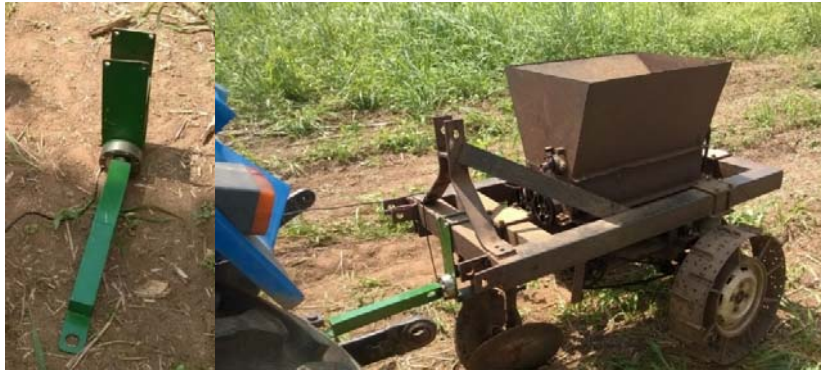
Fig. 4 Load Cell and Bracket as Installed on the Planter
