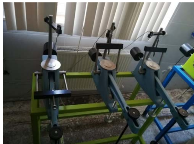
Fig. 1 Semi-automatic oedometer (consolidation) test machine used in the experiment
