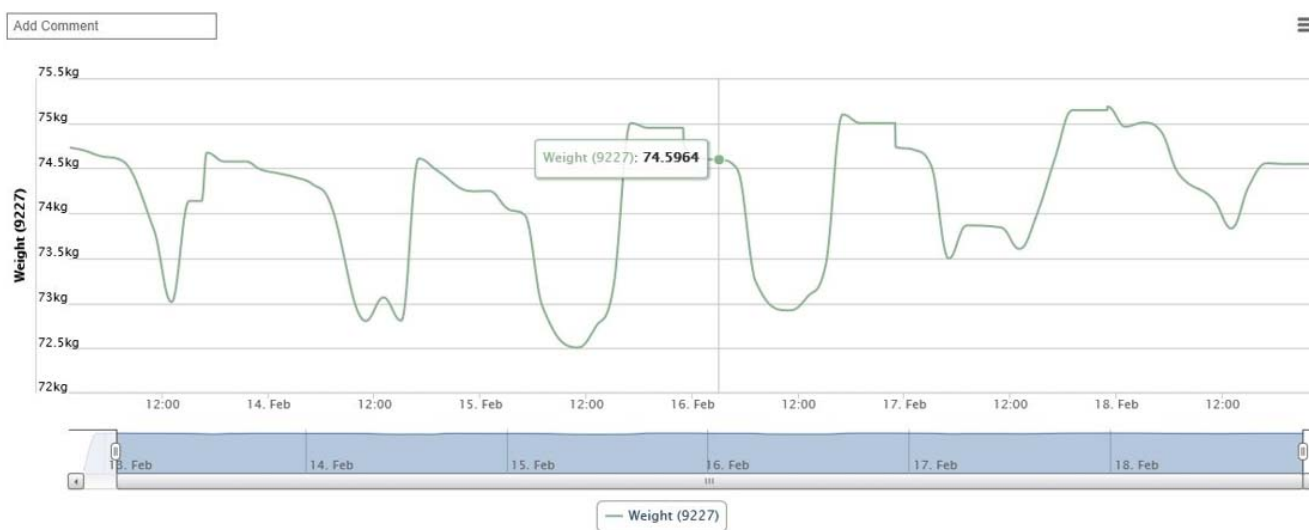
Fig. 1 Hive weight recording using automatic hive monitoring system: Weight data collected automatically from an active hive and transmitted to a website for review; Weight data can be collected in real-time for any number of hives and is easily interpreted for indications of activity and potential problems
