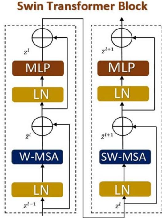
Fig. 4 Two Successive Swin Transformer Blocks with Multihead attention and Shifted Window Attention [32]
