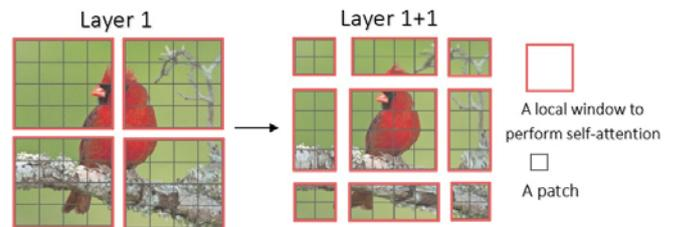
Fig. 3 Shifted-Window method to compute self-attention [32]
