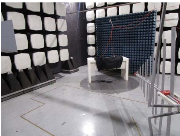
Fig. 2 The set-up of SAC for EMI radiated emission according to EN 55032 in Cetecom Essen, Germany
