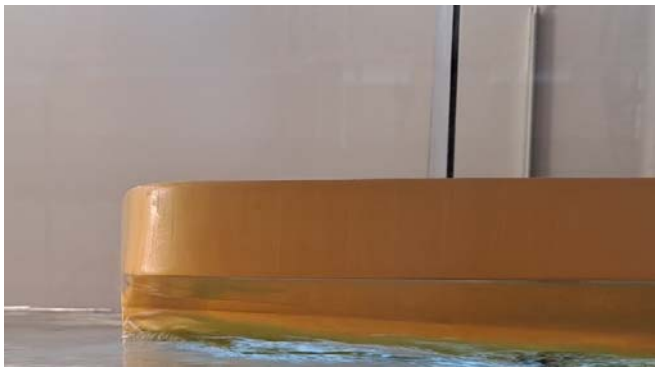
Fig. 5 Water flow at stem of the model at maximum test speed of 1.04 m/s
