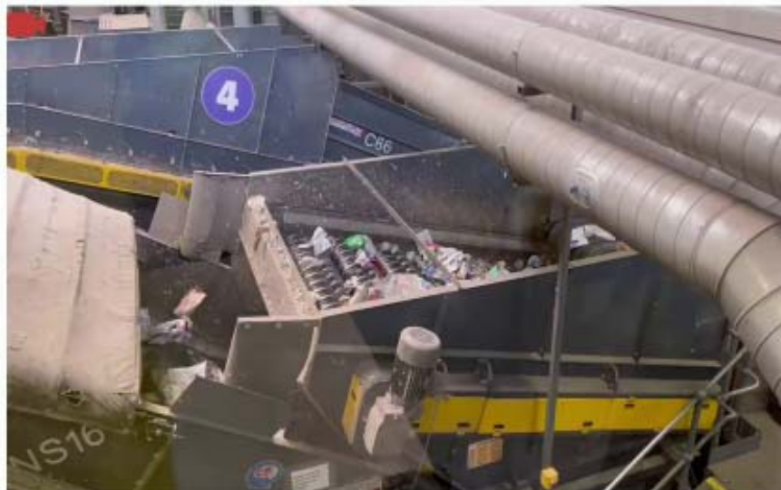
Fig. 5 Step 2), number 4: the glass separation process
