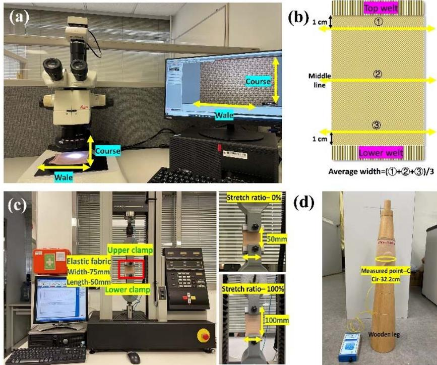
Fig. 2 Experimental investigations, (a) fabric density analysis, (b) fabric circumference test, (c) uniaxial Instron 4411 tension tester, and (d) fabric pressure testing
