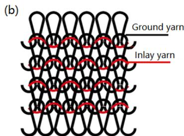
Fig. 1 (a) Characteristics of yarn materials, and (b) 1×1 laid-in knitted structure
