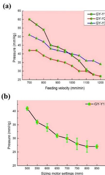
Fig. 3 Effects of machinery settings (a) feeding velocities and (b) sizing motor settings (loop sizes) on fabric pressure performances
