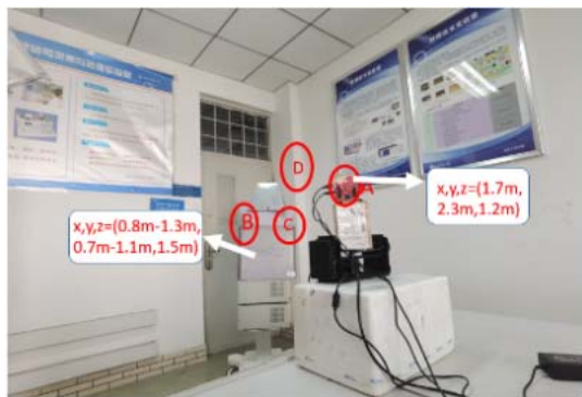
Fig. 7 (a) Distance calibration diagram
