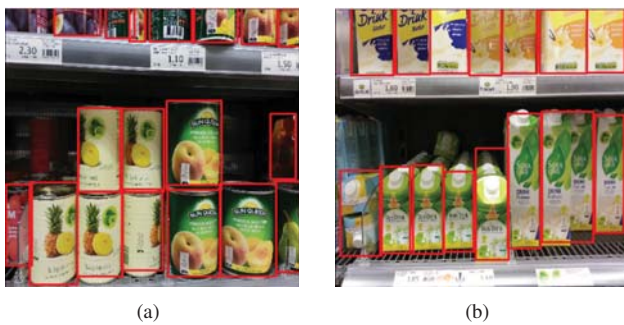
Fig. 5 Sample rack images from GP-180 and the bounding boxes predicted by our Faster-RCNN-based product detector marked in red
