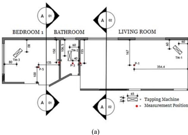
Fig. 3 Accelerometer and tapping machine positions on the apartment floor (P-1, P-3 and P-5) and walls (P-2 and P-4): (a) Floor plan; (b) Floor plan cuts (A<sub>1</sub> and A<sub>2</sub>)
