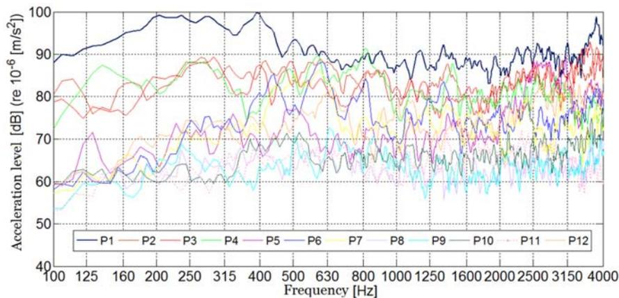
Fig. 7 Variation of floor acceleration level measured at distinct positions located in the apartment. The tapping machine location was fixed on the living room floor
