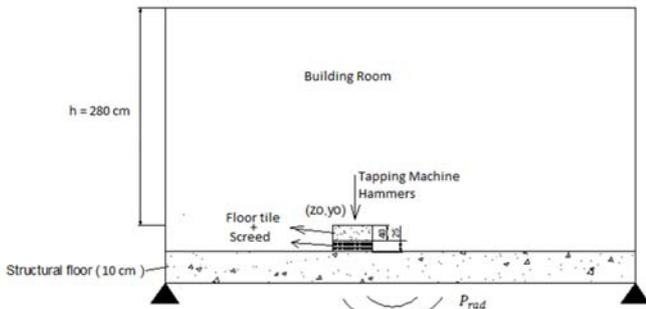
Fig. 1 Set-up of the experimental tests
