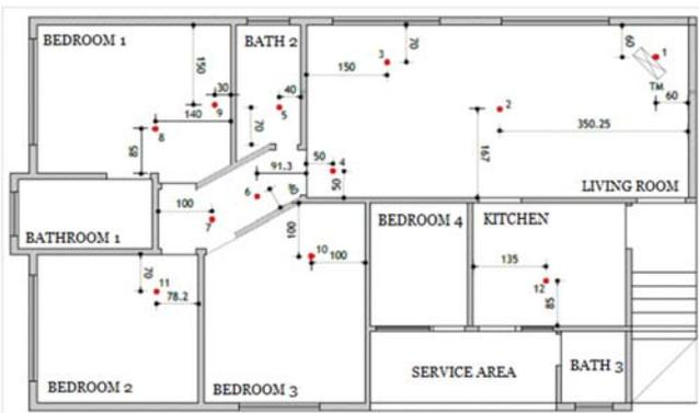
Fig. 2 Accelerometer positions on the apartment floor and tapping machine at position TM-1
