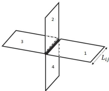
Fig. 4 Cross-junction type considered for the determination of the vibration reduction index  $K_{ij}$  between floors and walls: The subscripts  $i, j$  represent the source and receiver plate, respectively
