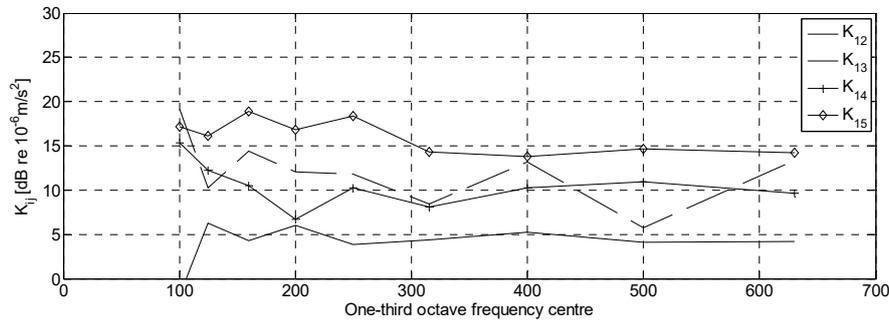
Fig. 8 Variation of the Vibration Reduction Index ( $K_{ij}$ ) with frequency and accelerometer positions P<sub>1</sub> - P<sub>5</sub>. Four different situations were considered:  $K_{12}$  (TM1 – P<sub>2</sub>),  $K_{13}$  (TM1 – P<sub>3</sub>),  $K_{14}$  (TM1 – P<sub>4</sub>) and  $K_{15}$  (TM1 – P<sub>5</sub>)
