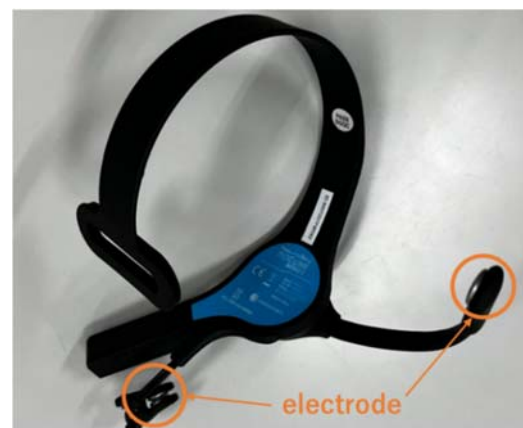
Fig. 6 Image of the simple EEG scanner (Mindwave MOBILE (Neurosky Ltd., CA, US))
