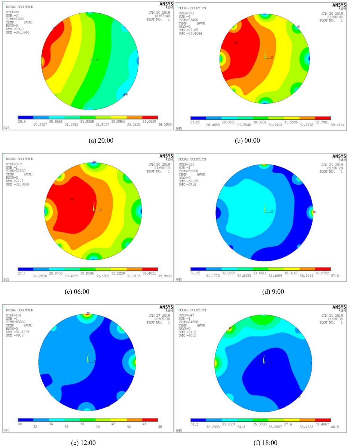
Fig. 6 Cross-section temperature distribution of main cable at each typical time
