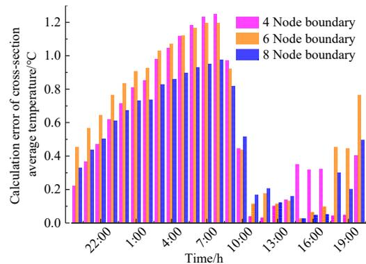
Fig. 9 Calculation error of different boundaries
