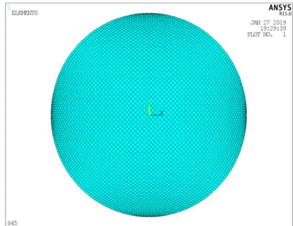
Fig. 5 Cross-section model of main cable
