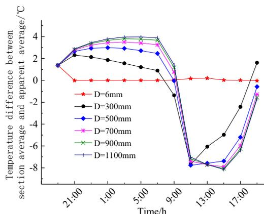
Fig. 11 Difference between sections with different diameters and apparent average temperature
