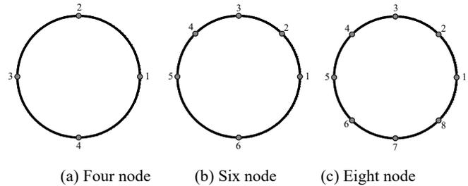
Fig. 8 Arrangement of main cable surface temperature measuring points
