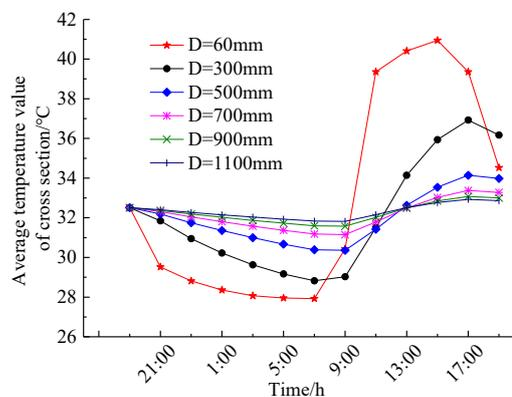
Fig. 10 Average temperature of main cables with different diameters
