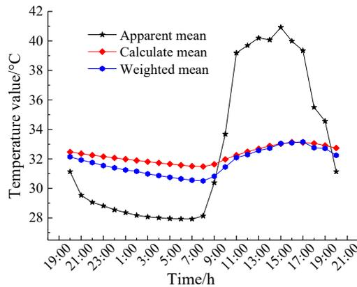
Fig. 7 Comparison of calculation results of three methods for section average temperature
