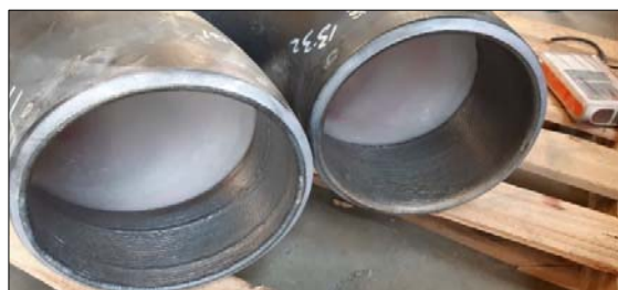
Fig. 6 Elbow transition cladding
