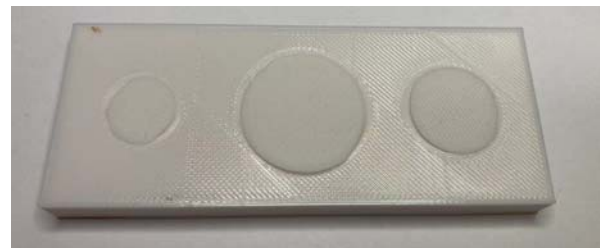
Fig. 8 The repaired faulty sample with the dents filled
