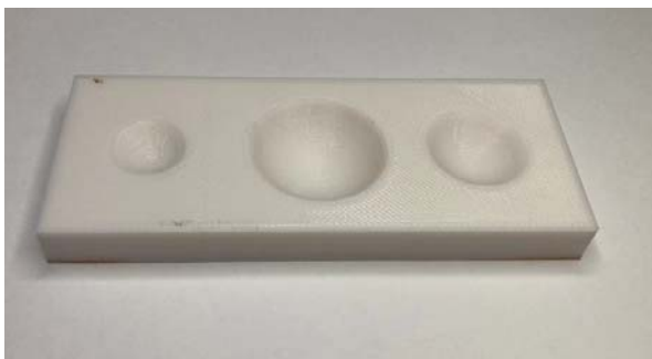
Fig. 1 (a) The 3D printed sample with proposed defects (dents)
