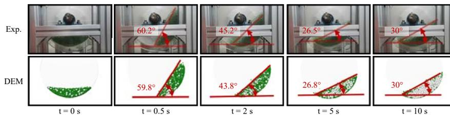
Fig. 4 Radial segregation image sequences ( $n = 40$  rpm,  $F = 10\%$ ).
