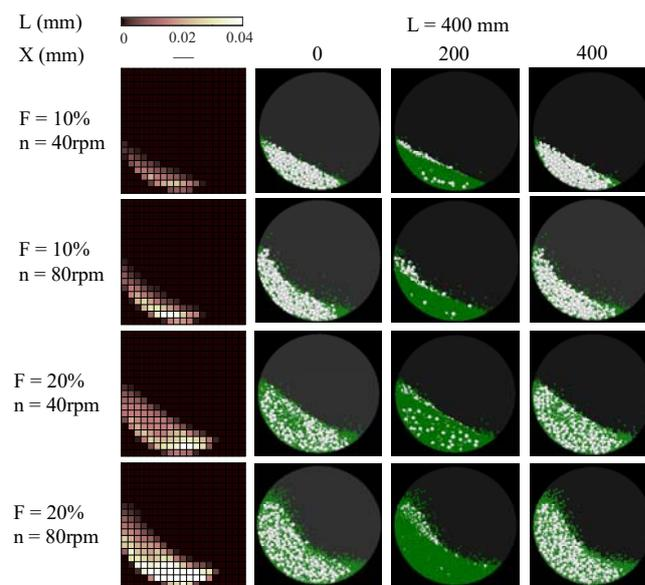
Fig. 7 Radial segregation pattern on the surface and inside of drum and its RRTE ( $t = 10$  s)
