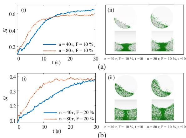
Fig. 6 The overall segregation degree  $SI$  under different conditions: (a)  $F = 10\%$ ,  $n = 40 - 80$  rpm, (b)  $F = 20\%$ ,  $n = 40 - 80$  rpm
