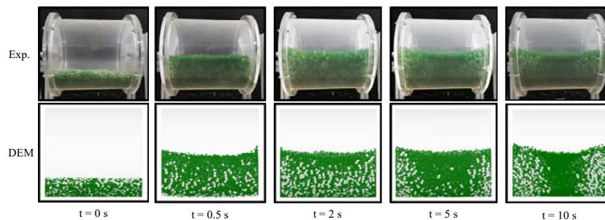
Fig. 5 Axial segregation image sequences ( $n = 40$  rpm,  $F = 10\%$ )
