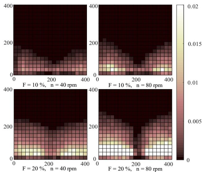
Fig. 8 Axial segregation pattern and its RRTE ( $t = 10$  s)
