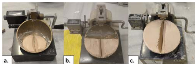
Fig. 4 Grooved soil paste for each placement form in the Casagrande cup: (a) under-filled, (b) half-filled, (c) full-filled
