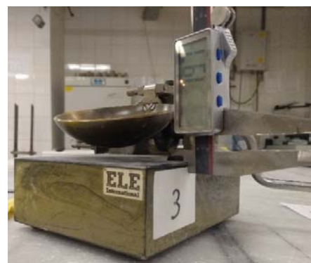
Fig. 2 Drop height calibration of the Casagrande device by a digital gauge
