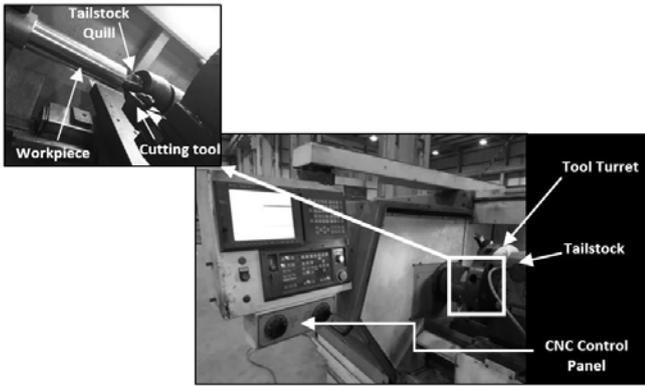
Fig. 2 Experimental set-up for 6060 Aluminium alloy turning trials
