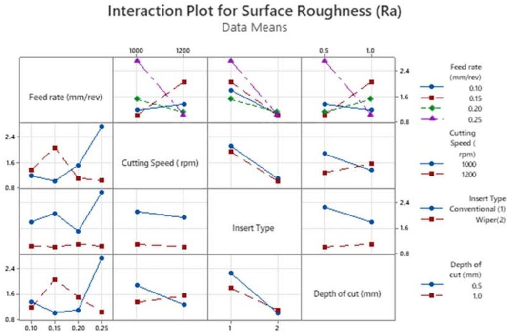
Fig. 8 Interaction effects of process parameters on average surface roughness (Ra)
