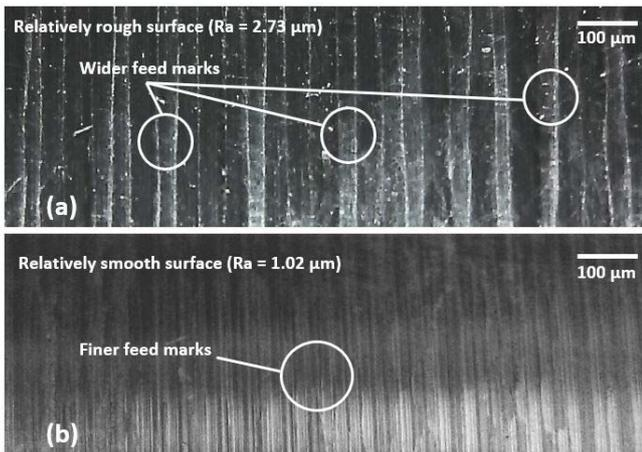
Fig. 7 Images of machined surface obtained at 1000 rpm cutting speed and 0.5 mm depth of cut for: (a) conventional insert (b) wiper insert
