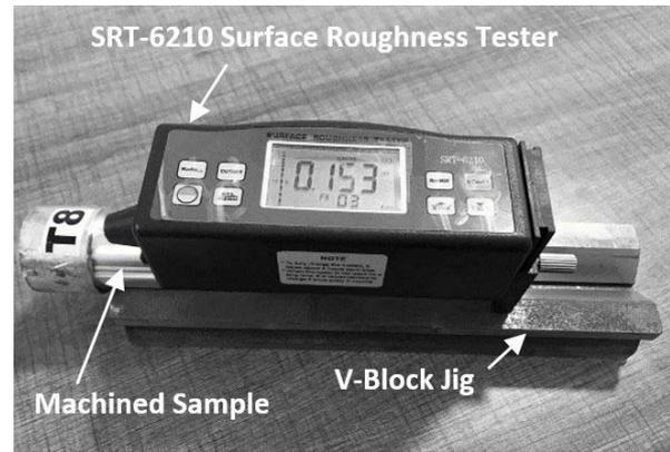
Fig. 5 Image of Ra measurement set-up used for the 6060 machined bars
