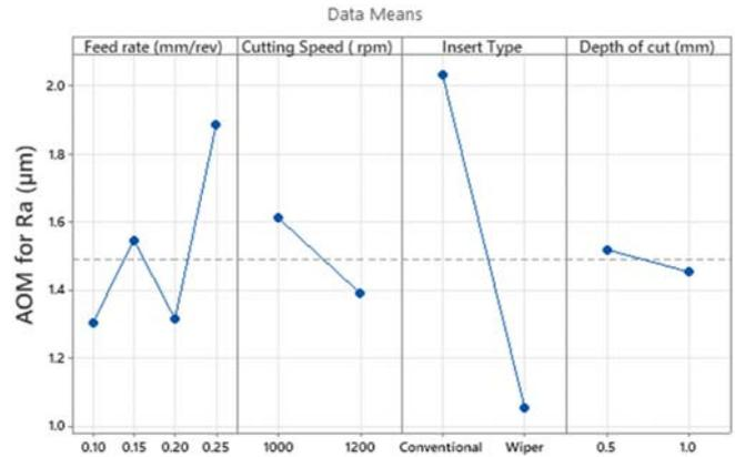
Fig. 6 AOM for average surface roughness (Ra)
