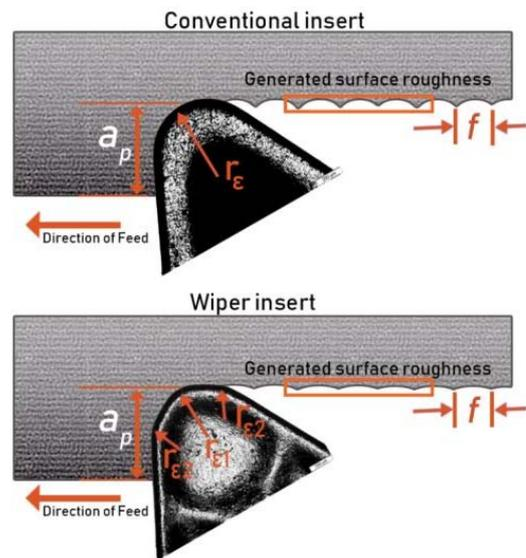
Fig. 1 Cutting mechanisms of conventional and wiper inserts [6]
